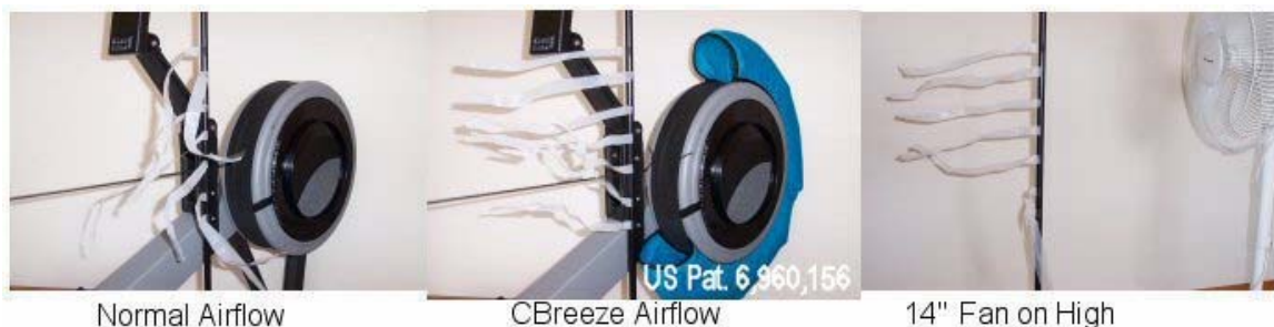
Figure 5. These pictures depict the concentrated airflow generated by the C Breeze. The inventor claims that this device can produce wind speeds greater than a 14" fan on high setting, however, this assertion seems disputable. It does do an adequate job of
